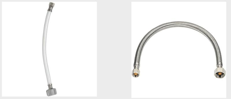
Soft, smooth plastic water lines shall be replaced with approved metallic lines in accordance to the International Plumbing Code. However, hard plastic water lines attached to the shut-off valve **at the factory** are allowable. White braided supply line is acceptable.
