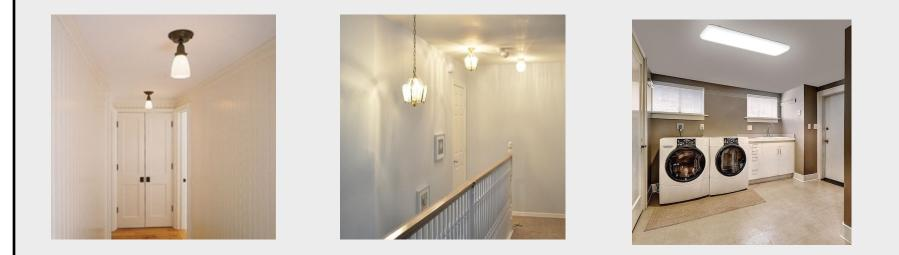
Every public hall, interior stairway, toilet room, kitchen, bathroom, laundry room, and furnace room shall contain at least one light fixture. Repair/replace broken fixtures.
