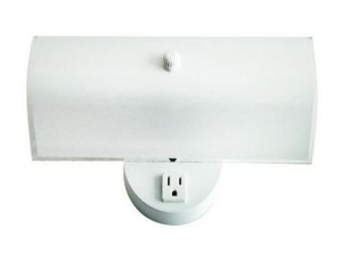
There must be at least one outlet in each bathroom. All receptacles in bathrooms must be GFCI protected. Outlets attached to light fixtures must be GFCI protected or removed.
